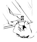
Tilt washer backward and remove corner post(s). Gently lower washer to floor.
